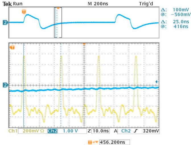
**Figure 7.8:** Close-up view of the second LVDS output channel that transmits data to the Cluster Processor. All data are zero for both MCM channels. A unit length in x direction corresponds to  $10\text{ ns}$ ,  $200\text{ mV}$  in y direction for the LVDS data, and  $1\text{ V}$  for the input signal. The zero line is indicated by the number 2 on the left side of the picture.
