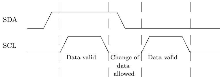
**Figure 6.10:** Bitwise data transfer on the I<sup>2</sup>C-bus.
