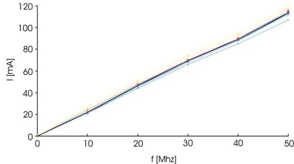
**Figure 7.2:** Current consumption of nine PPrASICs with applied RESET as a function of the clock frequency. Each line corresponds to a single chip. No analog input was applied.
