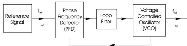
**Figure 5.3:** Scheme of a Phased Locked Loop (PLL).
