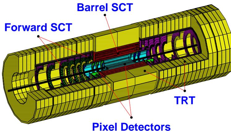
**Figure 2.5:** The Inner Detector of the ATLAS experiment [21].
