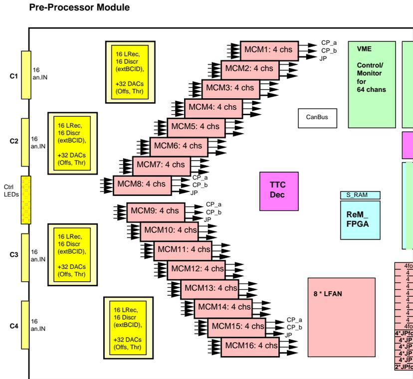
Figure 4.2: Layout of the Pre-Processor Module (PPM) [28].
