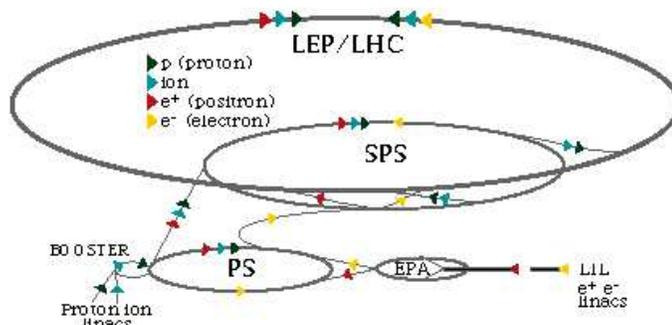
**Figure 2.1:** The accelerator chain at CERN [11].
