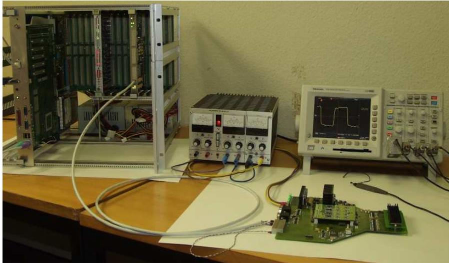
**Figure 5.9:** Photograph of the MCM test system.
