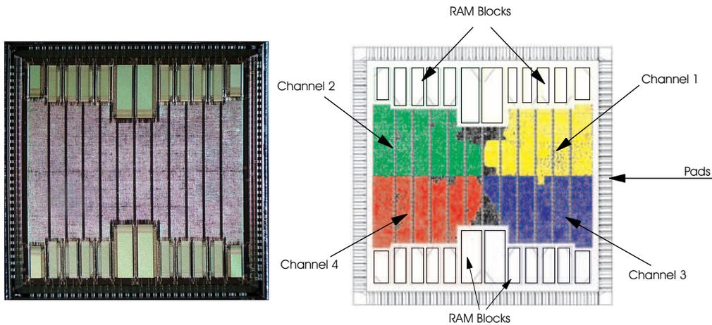
**Figure 4.6:** Photograph and Layout of the Pre-Processor ASIC (PPrASIC) [36].
