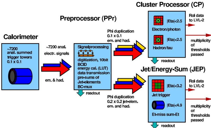
**Figure 3.3:** The calorimeter trigger with its three processors: the Pre-Processor, the Cluster Processor and the Jet/Energy-Sum Processor [12].
