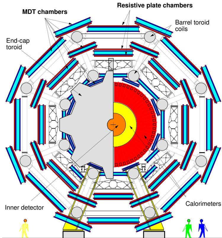
Figure 2.7: Cross-sectional view of the ATLAS muon spectrometer [22].
