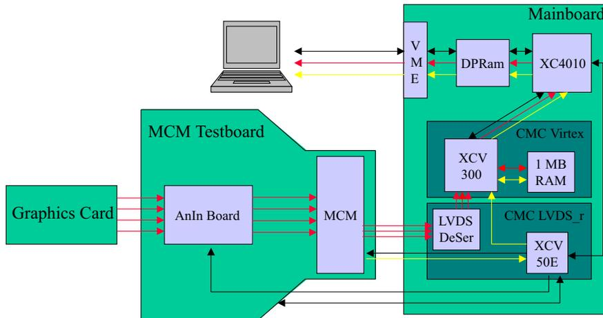
**Figure 5.8:** Block diagram of the MCM test system. The real-time data path is indicated in red, whereas the ReadOUT data path is illustrated in yellow. Configuration and setup data paths are shown in black.
