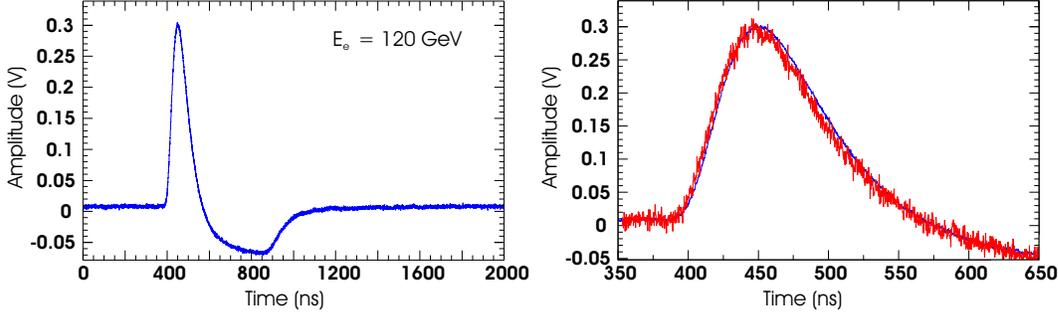
**Figure 6.1:** HEC calorimeter trigger tower test beam pulses. Left: Averaged signal of 120 *GeV* electrons. Right: same as left plus a single signal (red).
