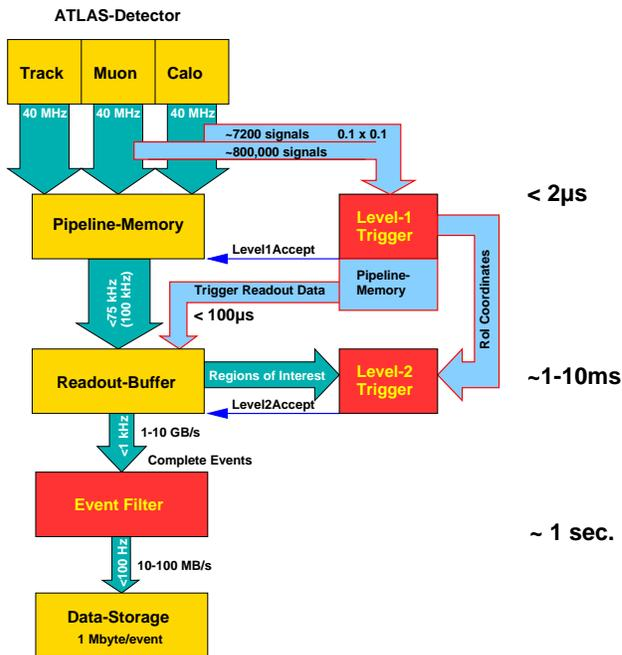
Figure 3.1: Detector read-out and trigger system [12].
