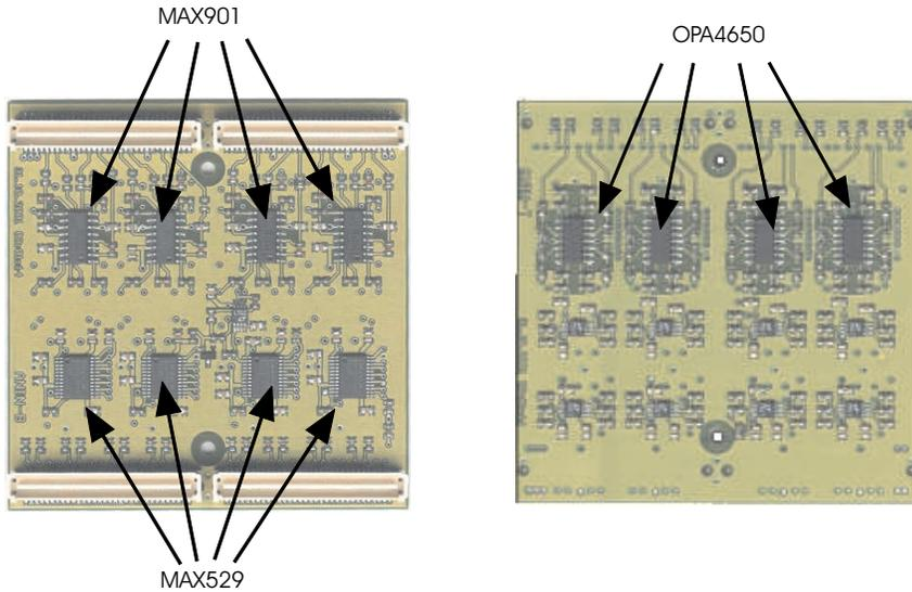
**Figure 4.3:** Photograph of the Analog Input Board.
