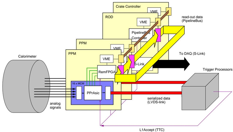
**Figure 4.1:** Block diagram of the readout configuration [23].
