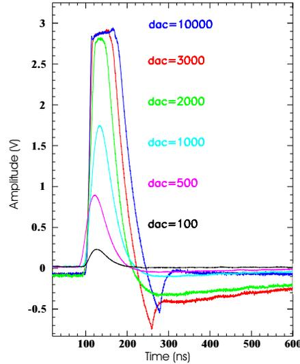
**Figure 6.2:** HEC calorimeter trigger tower calibration system pulses representing particle energies over the full dynamic range.
