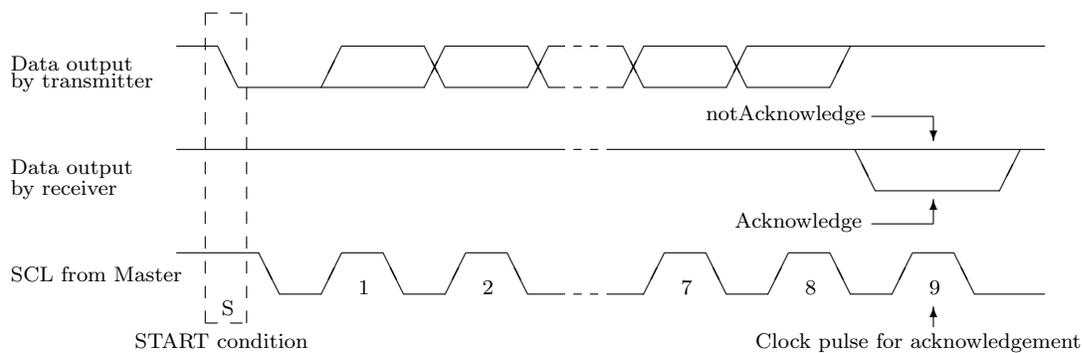
**Figure 6.11:** Acknowledge on the I<sup>2</sup>C-bus.
