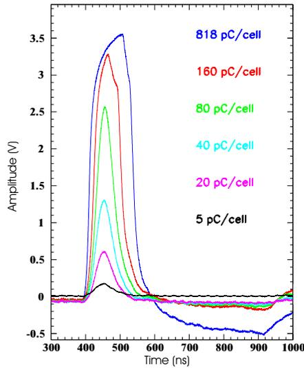
**Figure 6.4:** Hadronic tile calorimeter trigger tower pulses resulting from various injected calibration charges.
