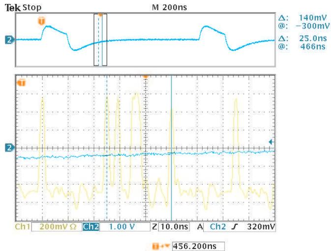
**Figure 7.6:** Close-up view of the BCID pattern generated by the PPrASIC as a consequence of the pulse shown in the upper part of the picture. These data are transmitted to the Jet/Energy-Sum Processor. The unit length in x direction corresponds to  $10\text{ ns}$ ,  $200\text{ mV}$  in y direction for the LVDS data, and  $1\text{ V}$  for the input signal. The zero line is indicated by the number 2 on the left side of the picture.
