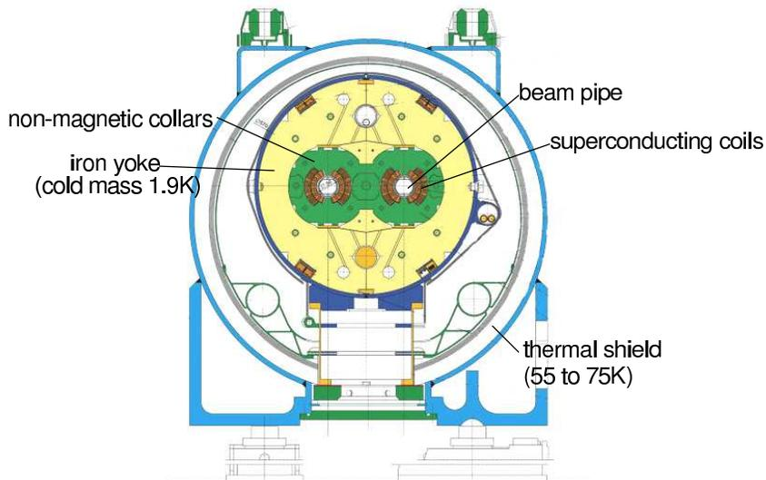
**Figure 2.3:** Cross-section of a LHC two-in-one dipole [18].
