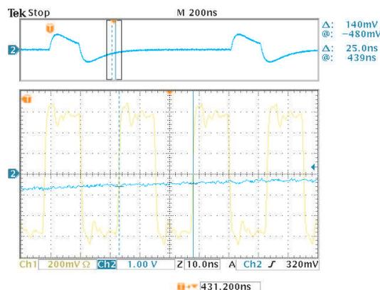
**Figure 7.3:** LVDS synchronization pattern (yellow) issued by the MCM LVDS serializers. A unit length in x direction corresponds to  $10 ns$ , whereas the unit length in y direction corresponds to  $200 mV$  for the LVDS data and  $1 V$  for the input signal. The zero line is indicated by the number 2 on the left side of the picture.
