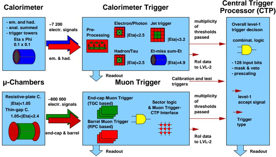
**Figure 3.2:** The ATLAS Level-1 Trigger system with its major components: the Calorimeter Trigger, the Muon Trigger, and the Central Trigger Processor [12].
