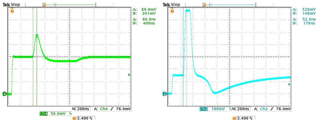
**Figure 6.5:** Simulation of HEC calorimeter test beam and calibration pulses. The unit length in x direction corresponds to  $200\text{ ns}$ , whereas the unit length in y direction corresponds to  $50\text{ mV}$  in the left picture and  $100\text{ mV}$  in the right picture. The zero line is indicated by the numbers 4 and 2, respectively, on the left side of each picture. Left: Test beam pulse caused by a  $120\text{ GeV}$  electron. Right: Saturated pulse.
