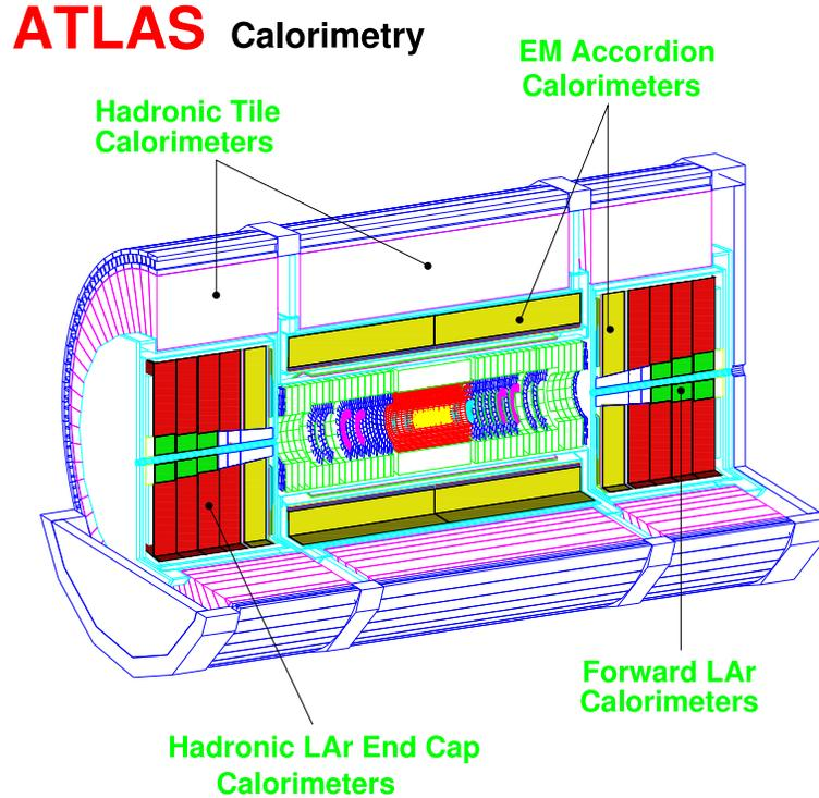
**Figure 2.6:** The ATLAS Calorimetry [19].
