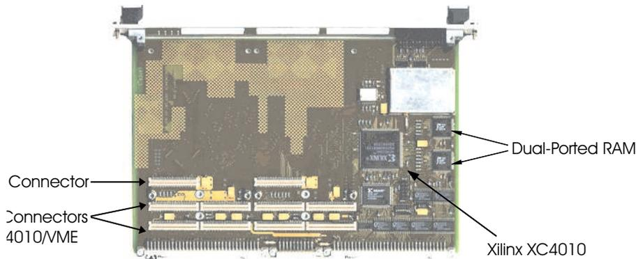
**Figure 5.5:** Photograph of the general purpose motherboard.
