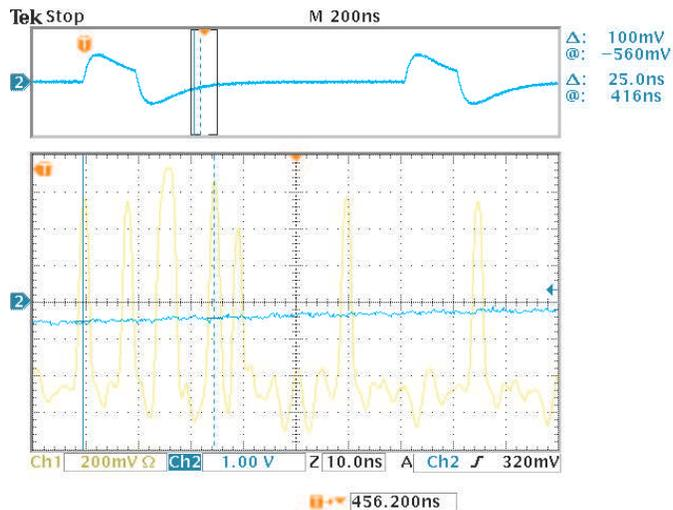
**Figure 7.7:** Close-up view of the LVDS output channel that sends non-zero data to the Cluster Processor. A unit length in x direction corresponds to  $10\text{ ns}$ ,  $200\text{ mV}$  in y direction for the LVDS data, and  $1\text{ V}$  for the input signal. The zero line is indicated by the number 2 on the left side of the picture.
