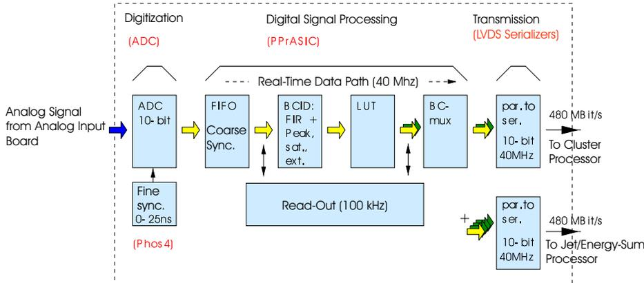
**Figure 4.5:** Block diagram of the signal processing within the MCM [37].
