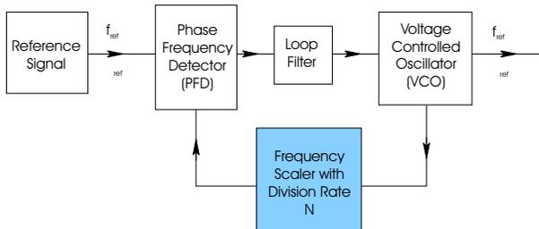
**Figure 5.4:** Scheme of a PLL with frequency scaler.
