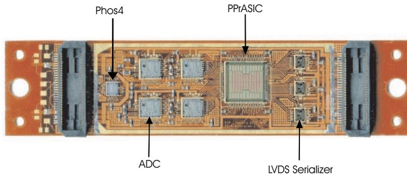
**Figure 4.4:** Photograph of the Pre-Processor Multi-Chip Module (MCM) [37].
