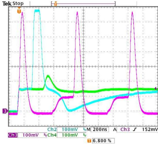
**Figure 6.6:** Simultaneous signal generation on all three color outputs. The unit length in x direction corresponds to  $200\text{ ns}$ , whereas the unit length in y direction corresponds to  $100\text{ mV}$ . The zero line is indicated by the number 3 on the left side of the picture.
