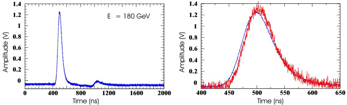
**Figure 6.3:** Hadronic tile calorimeter test beam pulses. Left: Averaged signal of 180 GeV pions. Right: same as left plus a single signal (red).
