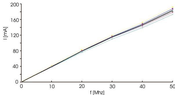
**Figure 7.1:** Current consumption of nine PPrASICs without RESET as a function of the clock frequency. Each line corresponds to a single chip. No analog input was applied.
