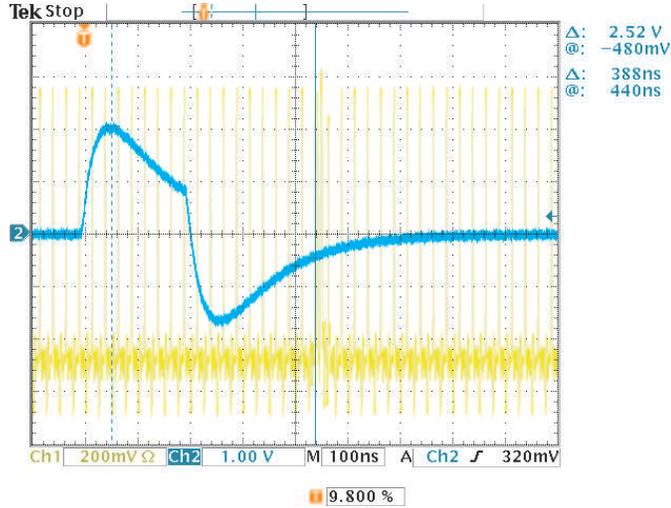
**Figure 7.5:** Analog input pulse and BCID output on the real-time Jet/Energy-Sum LVDS channel. A unit length in x direction corresponds to  $100\text{ ns}$ ,  $200\text{ mV}$  in y direction for the LVDS data and  $1\text{ V}$  for the analog input signal. The zero line is indicated by the number 2 on the left side of the picture.
