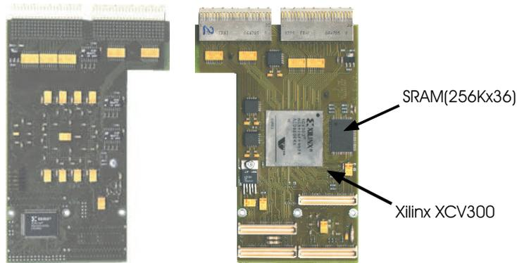
**Figure 5.7:** Photograph of the Virtex CMC.
