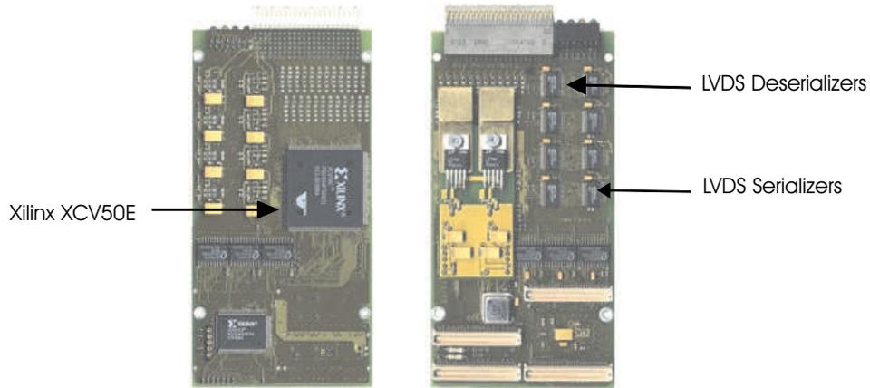
**Figure 5.6:** Photograph of the LVDS Receiver CMC.
