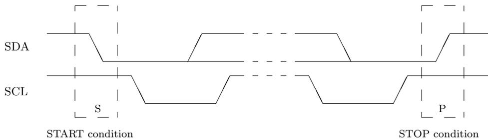
**Figure 6.9:** START and STOP conditions of the I<sup>2</sup>C protocol.
